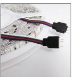
2) Insert the four pins on the side of the reel to the IR transformer. The arrows should be pointing toward each other.
