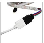
3) Connect AC power cord to the transformer. The lights should come on.
